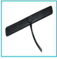
A small, low profile antenna for use where space is very limited, possible to glue to the underside of chamber lids. Can be attached with included adhesive strips of small fixings through premoulded holes.
